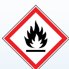
GHS 02 Flammable Self-reactive Pyrophoric liquids & solids Self-heating reactive Emit flammable gases Organic Peroxides
