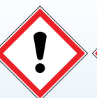
GHS 07 Acute toxicity Skin irritation Eye irritation Skin sensitisation Respiratory tract irritation Specific Target Organ Toxicity
