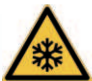
W010 - Warning: Low temperature/freezing conditions
