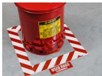
8. Colour-code hazardous areas or equipment.
